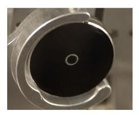
Double-mirror for pump-probe attosecond experiments. Tailored mirror coating for specific energy selection for reliable generation of isolated attosecond pulses.
